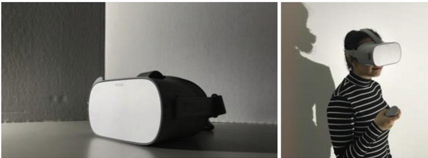
**FIGURE 7.2** The Oculus Go pictured here is an example of a head-mounted display (HMD), that is untethered (not attached to a computer) and also does not rely on a phone. Photos taken and edited by author Swati Pandita.
