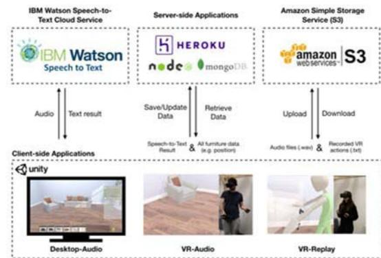
Figure 1: Prototype implementation under client-server architecture
